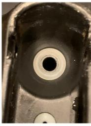
And finally, I snapped in the mouthpiece. All it now tight and the air leak is gone.
