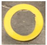
Using a leather punch for the outside diameter and a paper punch for the inside diameter, I cut out a spacer.
