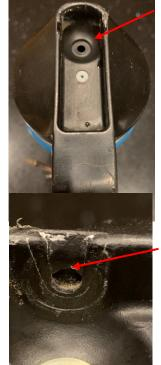
After cleaning out all remnants of mineral, I reassembled the Oring and mouthpiece. It leaked far worse than before!
