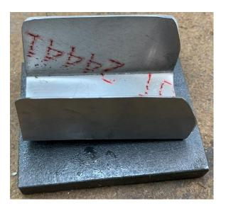
I bent up some tempered aluminum sheet stock and bolted it to a scrap of hot rolled steel. It was secured at one end with a 6-32 into a tapped hole. The other end has a longer 6-32 with a spacer to provide a slight angle. It too screwed into a tapped hole.
