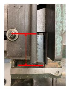
The length is set by the blade to movable jaw pivot bolt distance on the saw.
