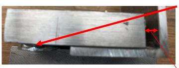
Note that the small bar sets the front floating jaw level as it contacts the back floating jaw.
