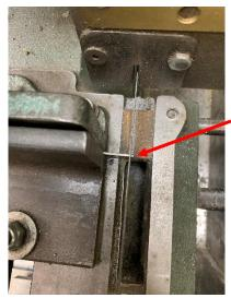
My 4 by 6 Horizontal/Vertical bandsaw is great for holding and cutting large stock. But when faced with cutting tiny bits of material, it needs some help. Those big jaws do not extend out to the blade so this thin stock tends to vibrate and bend due to the cutting force.
