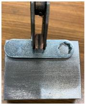
The front jaw is a block of metal the same length as the angle and 2 inches wide. It is ½ inch thick.
