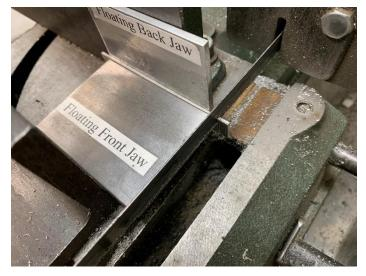
This long thin piece of stock is supported by the floating jaws right up to the blade.
