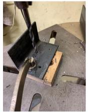
I located the second hole by eye. It should be "pleasingly close" but, again, the exact position is not important. Ultimately, this hole will also pass a lag screw.
