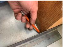
I started by slapping some angle stock against the first leg of the bench. I don't care about its cut length, just want it to match the leg. So a quick mark with a pencil is precision enough.
