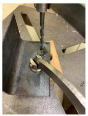
Moving over to my drill press, I drilled my first hole with a 3/16 bit. Eventually, this hole will pass one of two lag screws. The location of the hole looks about right but I couldn't tell you its exact position.
