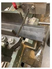
Then it's off to my bandsaw to cut off the piece. Note that the stock is placed with corner up. Assuming you are using a blade with at least 12 teeth per inch and with 1/8 inch thick stock, more than 4 teeth are in contact with the stock at the same time. This presents a constant amount of metal to the blade and, overall, saves time and stress on the blade.
