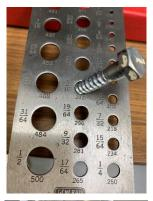
The next step was to rummage around in my selection of used lag screws and find two that were alike. Then I used my hole gage to find the closest fitting clearance hole, 5/16 of an inch. This will ensure minimal sliding of the angle stock around the screw when installed.
