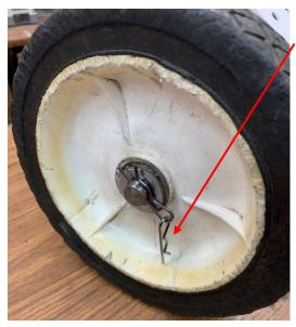
Each of my two wheels has *two* hitch pins. The loose pin on one wheel lets me pull the working pin without any drama. It is also the backup for the hitch pin on the other wheel.
