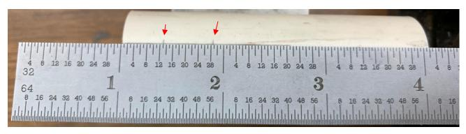
With the end of the pipe at the 1-inch mark and aligned with your pencil line, place a mark at 13/32. Make a second mark at 29/32.
