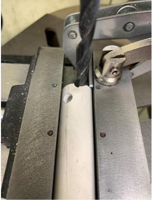
Rotate the pipe until the drill bit is no longer over the hole. If you have a way to measure this rotation, it is  $35^{\circ}$ .
