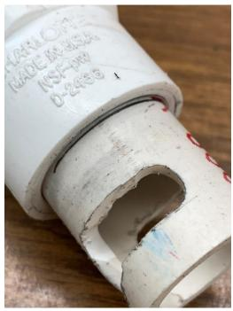
Press the bayonet into the threaded coupler until the line is barely visible.
