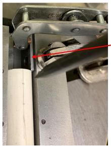
With the pencil line facing up, securely clamp the pipe in the vise. You will be drilling through, so be sure the gap in the vise is underneath.
