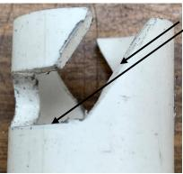
File only these edges of the pipe as necessary, so you clear the bar.
