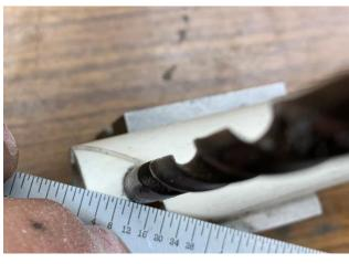
Insert the drill bit and draw a second line, parallel to the first, that is also tangent to the hole.
