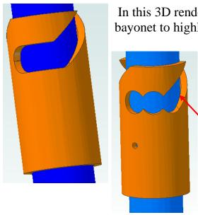
In this 3D rendering, I have placed an opaque cylinder inside the bayonet to highlight the finished cut.
