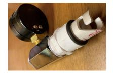
Here is the finished adapter. The compressor attaches to the Schrader valve on the top. The bayonet engages the Military valve at the bottom.
