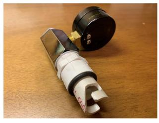
The bayonet is fragile, so I suggest you slide a coupler or end cap over it before placing the adapter in storage.
