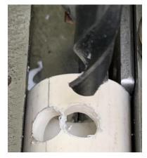
Rotate the pipe one more time (35°) and drill through for the third time.
