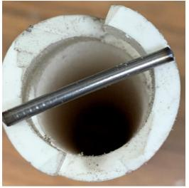
Using the outside diameter of the pipe as your gauge, cut the pointed end of the nail off, so you are left with a rod slightly shorter than the diameter. File off any burr.
