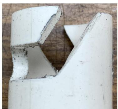
Using the Dremel cut-off wheel and your files, shape the PVC to this shape on both sides.
