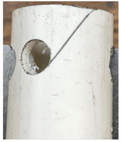
Remove the pipe from the vise and draw a tangent line from this last hole at approximately a 45° angle.
