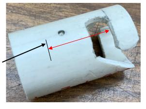
Draw a line 39/64-inches from the bottom edge of the finger, as shown here.
