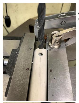
Chuck up the 17/64 drill bit and drill all the way through the pipe.
