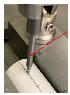
If you own a spud, use it to align the center of rotation of the drill press at the 13/32 tick mark. If not, you can use the smallest drill bit you own. Turn the chuck by hand and verify that the point of the drill bit does not wiggle off center. That would indicate that it is bent.
