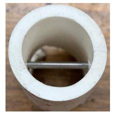
Install the rod in the pipe.
