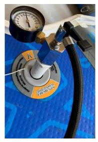
Attach your compressor. Lock the adapter to a Military valve and inflate to full pressure. If the threaded joint leaks, tighten another ¼ turn with wrenches and then retest. Over tightening will crack the plastic coupler. If the valve to O-ring contact area leaks, press the bayonet into the coupler a little more and retest.
