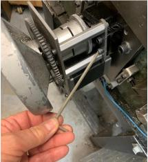
The long end lets me reach deep inside a machine to access a Socket Head Cap Screw.
