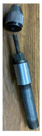
The chuck has a <sup>1</sup>/<sub>4</sub>-20 thread in the back. As the bolt mounted in the handle screws in, it pushes a disk which closes the jaws.
