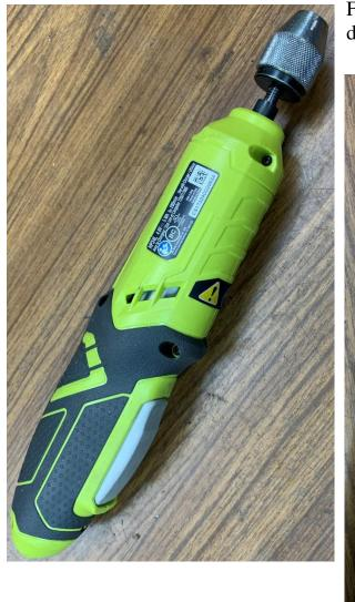
For light-duty work, it is handy to be able to drop a small drill chuck into a hex drive.
