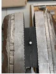
While steel vise jaws grip the sides of a piece of stock, rubber jaws wrap around it. This added support permits the user to apply
