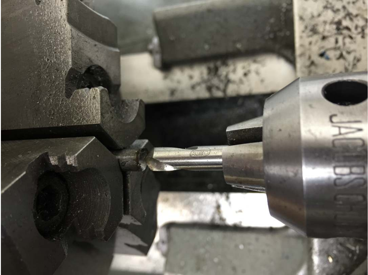
I used a \frac{1}{4} " spotting drill to form a cone shape hole. Note that this cone extends all the way out to the perimeter of the rod.
