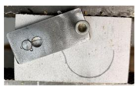
Then I dropped the guide into the hole and used the handle to rotate it until the line was centered in the hole. Then I drilled the next hole.
