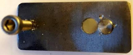
I drilled two 3/16-inch holes separated by 0.213-inches. This is the diameter of a #3 drill which I used as a spacer. Then I drilled and tapped a 6-32 hole to accept my little handle.
