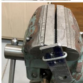
The ends of the wire go into my vise and I use the mandrel to twist the square loop.
