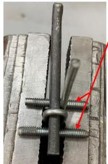
I then remove the clamping block and its bolts. Two lengths of threaded rod screw into the bolt holes.
