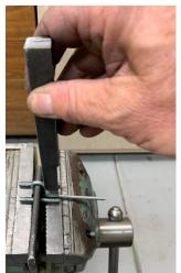
After tightening the vise, I'm ready for my next bend. I use the hammer to start the bend but then move on to tapping my steel bar to insure 90°.
