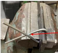
Again using my dead blow hammer, I bend the wire over as much as possible. Notice that the wire is angled so it bends past the first wire end.
