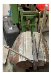
The mandrel is flipped over in preparation for bending the other end of the wire.
