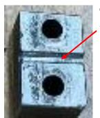
The clamping block has a tunnel across its face to secure the wire.
