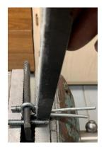
I again use the hammer to start the bend and the steel bar to finish it.
