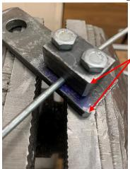
The clamping block with wire is secured to the mandrel with the two bolts.
