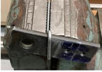
A gentle twist brings the wire ends into alignment.
