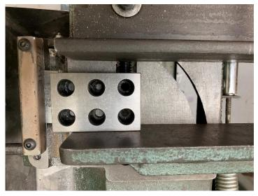
Recently I wanted to set the fixed jaw on my bandsaw perpendicular to the blade<sup>2</sup>. I pressed the jaw against a 1-2-3 block and then tightened the jaw's screws. Rechecking the alignment, it was clear that the jaw had moved. Hmm. I'd see this behavior before.
