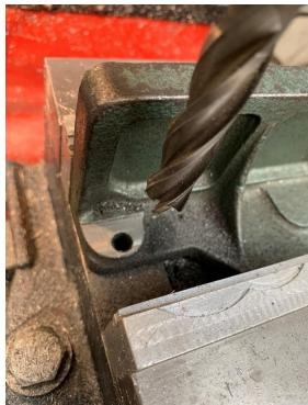
A few passes on my mill cut a surface parallel to the bottom of the jaw's flange around each screw hole.
