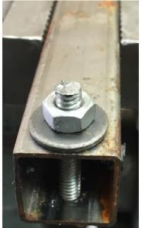
I took some threaded rod and screwed it into the hole. A thick washer and nut was installed on top. Then I used my torque wrench to see when it would tear out.
