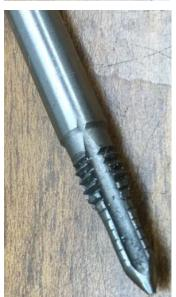
The goal is to form a hole that can be tapped. That is easy - freehand grind off the threads until only the root is exposed. I also ground the end to a point. Previous experiments showed that if the end is flat, a disk of metal is left in the bottom of the hole. That is wasted metal that can't be used in the walls of the hole.
