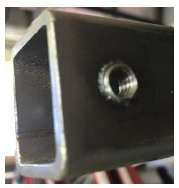
Is it possible to friction form a boss in steel tubing in order to increase the number of threads cut? Yup, with certain limitations.
