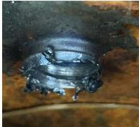
The underside tells a different story. The wall thickness is paper thin. So how good are these threads anyway?
