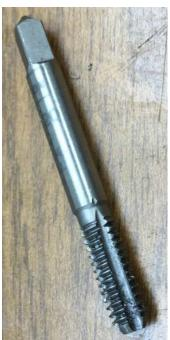
I started with a worn out 1/4-20 tap made of High Speed Steel.
