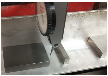
I then had room to rotate my fDTI by turning the spindle almost exactly 180°.
