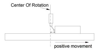
With the finger's contact point to COR known, I can go back to my original application. When the fDTI reads 0 and is contacting the block, the COR is 0.148 inches more negative.
