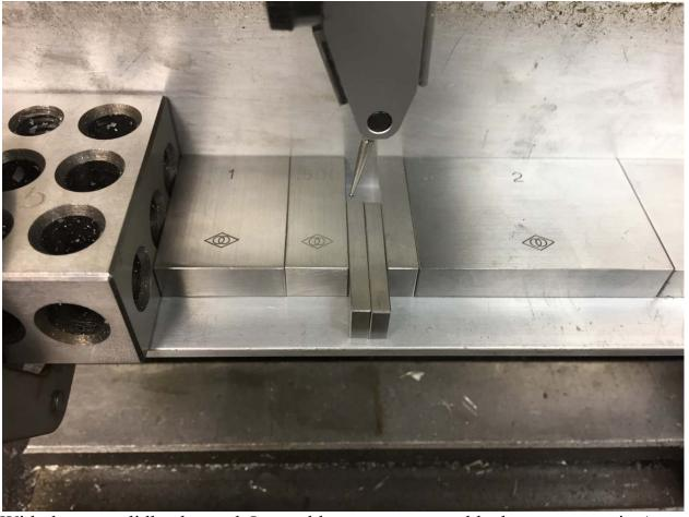
With the gap solidly clamped, I was able to use my gage blocks to measure it. A stack 0.295 inches thick just fit. 0.296 did not fit. This means that the COR is  $\frac{0.295 \ inches}{2} = 0.148 \ inches$  from the contact point of the finger. I am only entitled to 3 place accuracy and since the gap is between 0.295 and 0.296 inches wide, I rounded up.
