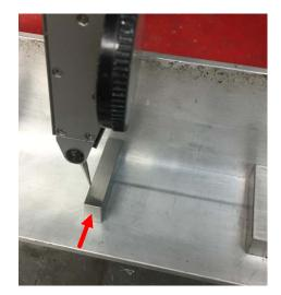
After zeroing my fDTI, I pushed on the end of that small block (red arrow) and removed the larger block to its right. Then I carefully slid the small block to the right. The goal was to not bump the finger.
