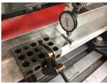
Next I slid a few blocks into the fDTI backed up by a 123 block from the left. I stopped when the fDTI again read zero. Then I clamped the 123 block.
