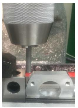
I mounted a piece of .250" drill rod in my drill chuck. In hindsight, I should have used a collet which has less runout.
