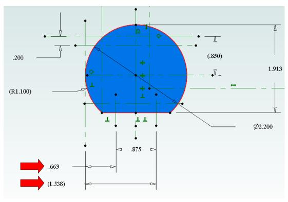
Since the part was drawn using CAD, I had access to all dimensions. The two key values are the distance from the perimeter to each of the hole centers: .663 and 1.538.
