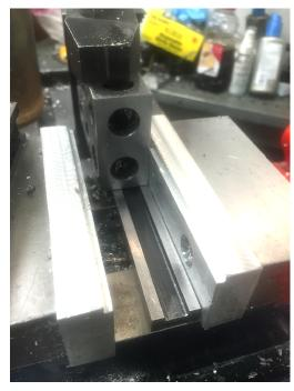
I started by placing a parallel down on my vise ways. Then I loosely clamped a 1-2-3 block on one end. The vise was lightly tightened to align the block. Then the hold down clamp was tightened.
