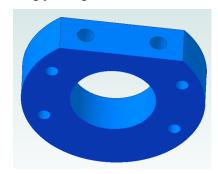
The challenge was to drill two holes in a flat that are within  $\pm .002$ " of their designed locations.
