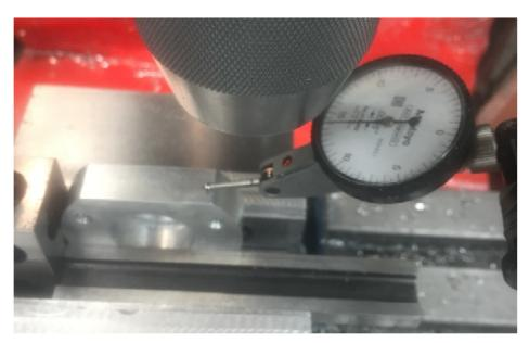
Then I moved the table so the finger was on the right side of the flat. The needled moved 0.014".
