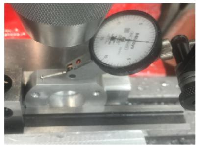
Next I mounted my finger Dial Test Indicator in my drill chuck. I zeroed it on the left side of the flat.
