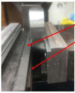
The part was placed on top of the bottom parallel and touching the 1-2-3 block's vertical face.
