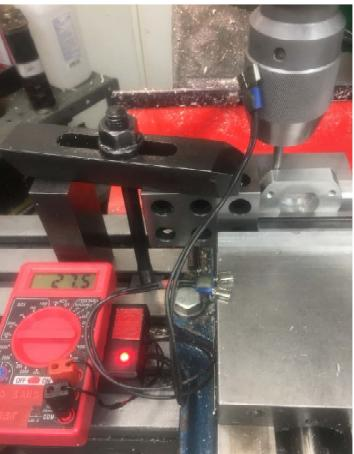
I used the same procedure to pick up my Y axis zero. This time the rod touched the back of the part.
