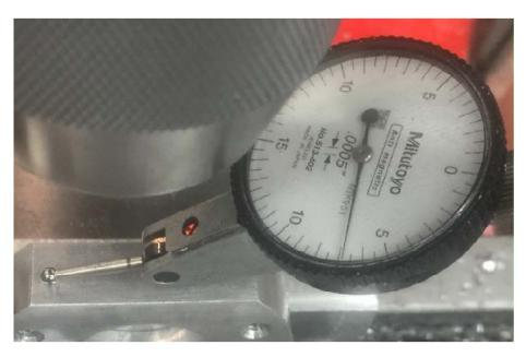
Going back to the left side of the flat the needle didn't move. The vise was then tightened.
