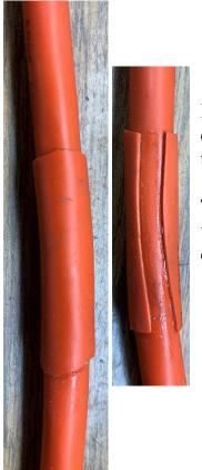
I centered the patch over the nick and wrapped it around the cord. A layer of thin steel wire wrapped around the path applied the necessary pressure. Wait the full curing time.
