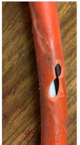
If just the outer sheath of a round cross-section extension cord has been nicked, people often wrap it in electrical tape. It looks good for a while but before long, the tape starts to lift. Bending of the cord loosens the wrap and dirt gets in. Before long, the entire mess falls off. Then you are back to having that exposed nick plus all of this sticky goo mixed with dirt around it. New tape won't stick to that. Gotta be a better way.
