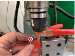
Using a non-rotating Electronic Edge Finder and the procedure presented here, it is possible to measure the distance between COR and a reference surface with an error much smaller than the repeatability of my milling machine.
