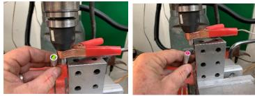
Proceed with finding zero on the X and Y axes. Always turn the spindle so the *A* reference mark faces the reference surface. If the probe is removed from the spindle, reinstall with the colored dots lining up.
