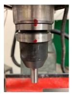
For some milling machine<sup>2</sup> operations, the Center Of Rotation (COR) of the spindle must be known relative to some reference surface attached to the table. This measurement can be done with a non-rotating Electronic Edge Finder<sup>3</sup> (EEF). Read on for a procedure that minimizes error due to run-out.
