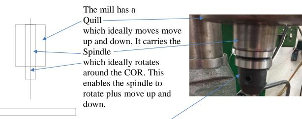
Attached to the bottom of the spindle is a means<sup>10</sup> by which cylinders like EEFs and cutters can be attached. Ideally, they attach in perfect alignment with the COR.
