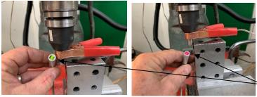
I was setting zero on my X-axis. The spindle was rotated so the *A* reference mark faced the reference surface, my 123 block. Then I had the CNC program automatically feed in until touchdown. Note that the LED changed from green to red.
