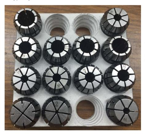
This ER-20 collet holder plate took just a few minutes to make using some expanded PVC board<sup>2</sup> and a drill press.
