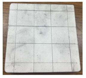
Starting with a piece of PVC board 3.5 inches wide, I cut off a 3.5 inches length. The lines are 0.9 inches on center and 0.4 inches from the outer edges.
