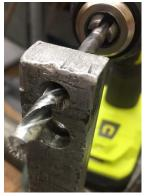
Poke the drill through your new drill guide with the countersunk side facing towards the point of the drill.
