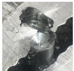
Here you see the top of the rivet almost cut off. I did have to adjust my drilling angle to stay centered but
