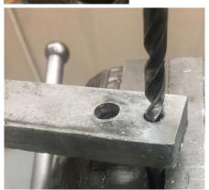
Place the assembly over the rivet head and adjust the top face of the guide so it is perpendicular to its major axis. You are now centered.
