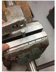
This drill guide works equally well on the end of a rod.
