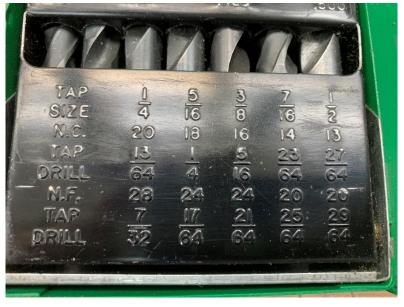
Then the solution just about jumped out of the index box — sand off the paint from the raised numbers. I used a very fine emery cloth. At first I put a block behind it but that wasn't necessary.
