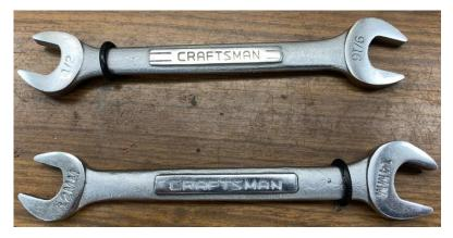
My solution is to stretch an O-ring over one end. This ring is tight enough to not freely slide over the raised logo in the center of the tool. The end with the ring nearby is the one that I do not want.
