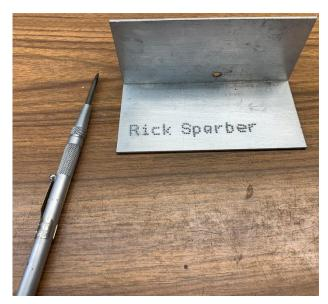
My "printer" consists of a layout punch. For deeper characters, I would use my marking punch.
