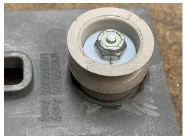
I'm using a nickel-plated flat head screw and a nickel-plated nylon lined lock nut. These will be replaced with stainless before they start to rust.
