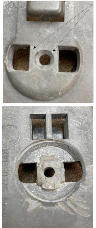
The first step was to scribe lines between the two cut-out areas in order to locate my new mounting hole. Then I used my 1/8" spotting drill at the intersection and followed with a #27 to give me a 6-32 clearance hole. Using a countersink mounted in a brace-and-bit, I carefully cut the recess. The screw must be flush with the surface to avoid binding. Fortunately, there is enough thickness to sink the screw head and still have strength.
