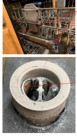
The weak links on my KitchenAide dishwasher are the wheels that carry the top rack. The wheel carrier is made of resin plastic which holds up well to the hot water but is brittle. This video explains the problem and how to replace the carrier: https://www.youtube.com/watch?v=TCC6gTu3un0
