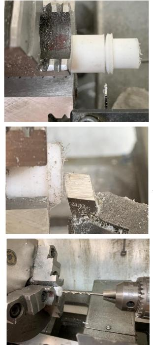
I took the dimensions from the spacer and turned the new axle. Here you see the overall length complete along with the outside diameter of the axle. I parted off with my hacksaw blade grooving tool<sup>2</sup>. The nylon squirms so I ended up with a crowned top.
