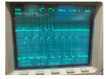
I can use my oscilloscope to look at the signal at a given General Purpose Input Output (GPIO) pin. I trust this information as long as its highest frequency does not exceed the capability of the 'scope.
