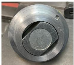
The length of the smaller OD permits about 10 thou of the Magswitch to be proud. This is necessary for maximum holding force.
