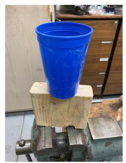
Here is my proof of concept. Just a block of 2 by 6 with a heavy plastic cup attached with two screws. I did sand the block to remove splinters but that was the extent of the refinements.
