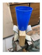
After using the cup holder for a few weeks, I have added two design elements. The first was these curved braces to the flanks of the block of wood. There were cut from 6-inch diameter ABS pipe. All edges were rounded. My inner thighs fit into these curved surfaces and greatly reduce the tendency of the cup to tilt on tight turns.
