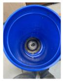
The second addition was to place a large washer in the bottom of the cup and secure it with a wood screw. This reduces the flexing of the cup during turns. The result is a more stable holder for my morning mug of coffee.
