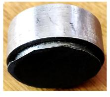
My solution was to use double-sided tape to attach a disk of 600 grit emery cloth to the bottom of the disk. This roughness is enough to prevent sliding while using a gentle holding force from my fingers.
