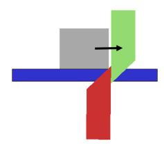
When the paper sheers, the bottom blade has jacked the top blade away from the disk. The result is a jagged edge on the paper. The cut starts on the arc defined by the disk but drifts off of it on each snip.
