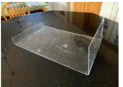
My solution consists of a sheet of 0.08-inch thick acrylic plastic. It is as wide as the opening at the door and as long as the distance from the right side of the door opening to the back wall of my Bermuda Triangle. Using a heat gun, I bent up a 7 inch tall stop on one end and a 2-inch tall lip on the other.
