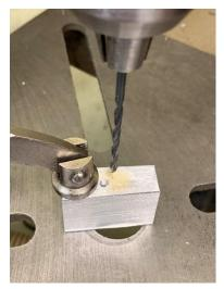
Next, I positioned my part and put the tap drill in my drill press chuck.
