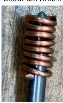
After trimming the ends, I slid the coil up to cover the square part of the shank.
