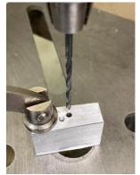
The best time to run a tap is right after the tap hole has been drilled. All is in alignment, and the chuck can drive the tap. Well, almost true.
