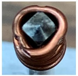
Can we relax the requirement a bit? Using some copper wire, I was able to form it close enough to transmit rotational force and be reasonably well centered.
