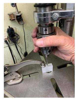
After introducing some tapping fluid into the hole, I fed the quill down with one hand until it contacted the part. I then used the other hand to turn the chuck one revolution. The tap was then bedded enough to counteract the upward force of the quill retraction spring. It was then easy to turn the chuck and cut the threads with one hand.
