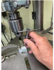
You may quickly run into problems. The tap, mounted in its handle, can't fit between the chuck and the part.
