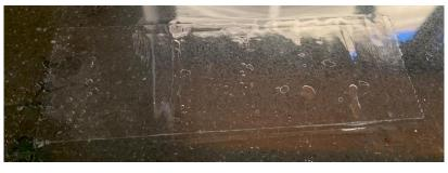
For my second test, I took a clean plate of glass and sprayed it lightly with water. Then I laid the tape, sticky side up, on the water.
