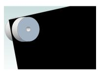
Most filing buttons are cylinders that bolt onto stock. By following the surface of a button, a person can file a curved surface that matches all or part of the cylinder's surface. The one thing that always bothered me about these buttons is that they require a hole for the bolt.
