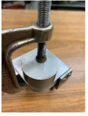
Karl\_H of homemadetools.net had an excellent question: how did I made the radius on the base? I took a piece of round stock 1¼" in diameter and clamped it to the base. Then I used a grinder followed by my belt sander to form the rounded corner on the base. So to make a button, you need a button. Thanks Karl.
