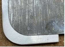
After deburring, the corner of the stock is a good approximation of a 7/8<sup>th</sup> inch radius.
