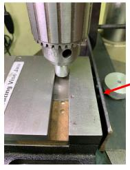
With a piece of 5/8 strap in my drill press vise, I installed the 5/8 tool in my chuck. Just lowered the chuck down until the tool entered the gap. Locked the vise in place and I was centered.
