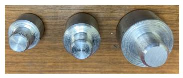
Each tool is made from aluminum round stock with the end turned down to about 3/8-inch.
