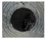
I had previously faced this piece in my lathe, and you can see a series of concentric circles that confirm the hole is centered fairly well. The hole should be as well centered as the point of the ½-inch drill.
