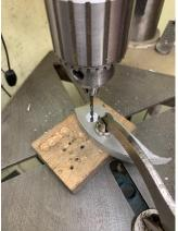
Next, I chuck up a 1/8<sup>th</sup> inch drill. Using the bottom of the cone for alignment<sup>2</sup>, I drill through. The custom tool is done.
