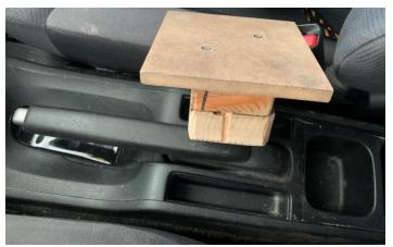
My solution was to build a table. Two chunks of scrap pine were glued together and shaped to fit the recess. The tabletop is a piece of scrap MDF held in place with two screws. Call this a "proof of concept," but I see no need to make it prettier.
