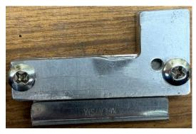
I collaborated with many readers during this development. After reading their insights, I built this version of the cable sheath stripper.
