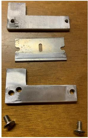
The cutter is a sandwich made up of a bottom, threaded plate, the razor, a matching top plate with through holes, and two 6-32 screws. The plates were sized to permit the razor to extend out no more than 0.025 inches.
