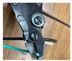
An excellent design stands the test of time. I've had these wire strippers for many decades. When adjusted correctly, it cuts through almost all of the insulation but does not touch the conductor. By pulling along the wire, the remaining insulation is torn through.
