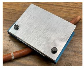
With input from Doug Lough, the design quickly evolved to be safer and able to accommodate a range of cable diameters. The two box cutter blades have been replaced by a razor blade which extends beyond the edges of the plates by a little less than the thickness of the sheath.
