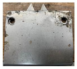
The sheet metal goes on next. It provides a stop, so the blades don't slide out the bottom as they are being adjusted. A lip on the bottom edge of the plate would do the same job.
