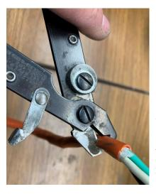
Yes, there are limits to this range. Trying to strip off the sheath of a cable tends to nick the wires inside. Yet, the basic idea of a V-shaped cutter is still a great idea. I just need to extend it.
