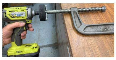
With the crossbar approximately centered, I push my "Speed Drive" against the end of the threaded rod. By slowly pulling the trigger, the clamp quickly adjusts to the desired position.
