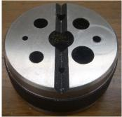
I had a backup plan involving the sawing of a V into the face of the puck. The V would grab the crossbar better but would mean that the user must first align the V to the bar. I'm glad I didn't need to do that. The fussier the tool, the less I use it.
