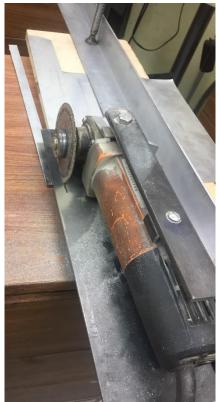
Power up the grinder and slowly pull it *towards* you. This should be a smooth, controlled action. Be sure to keep the support plate in contact with the fence.
