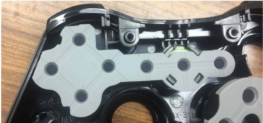
The dark grey dots face towards you. As with everything else, it is keyed so can only go on one way.
