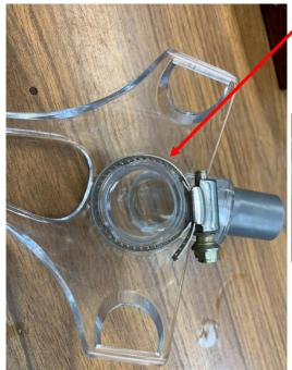
I tightened a hose clamp around the flange and warmed the plastic with my hot air gun. Then I quickly cooled it with a spray of distilled water.
