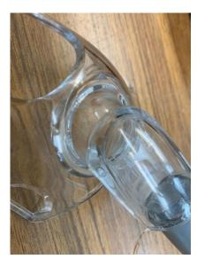
This holder is considered worn out when air leaks around this pivoting coupler.
