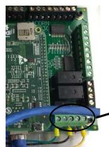
If you have a voltmeter, measure the voltage at the Acorn's H9 terminal block.
