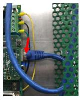
Since it is relatively easy to do, first power down the system. Then unplug each end of the cable and plug it back in. There is a catch (red arrow) that must be released before you can slide the plug out. When sliding the plug back in, listen for the click as the catch engages.
