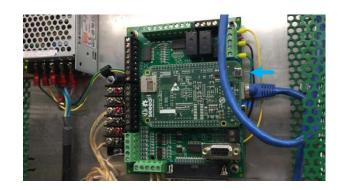
the Acorn software is running and ready to accept messages from the PC, this light will cycle on and off once a second. If you see other lights on but the blue light is not cycling on and off, something is wrong with the hardware or software of the Acorn<sup>5</sup>.
