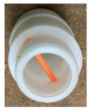
Looking inside, you can see an orange rod. This rod pushes down on the plunger within the Military valve to open it.
