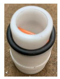
An O-ring fits over the small diameter and provides a seal. Given the low pressure, this is effective.
