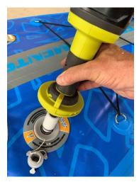
Here you see the adapter installed on the Ryobi in the deflated configuration. It is so effective that if I push on the button when done, air rushes *in*.
