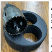
Both rubber plugs were dried out and cracked. Not to worry, I cut new ones with my hole saw and my ready supply of hockey pucks. I misjudged the height of one of the pucks so I had to make up for it on the other puck. This should not affect the operation of the bolt cutter.
