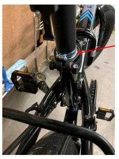
In preparation for using my bike stand, I installed a Dollar Store hose clamp around the seat post. The screw mechanism is aligned with the gap in the seat post clamp.
