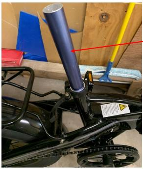
With the seat removed, I slide in my length of pool brush handle until it touches the floor. I had previously cut the top off, so about eight inches are exposed. Using a file, I removed the sharp edges.
