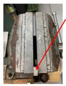
Sometimes I need to clamp a piece of stock at the end of my bench vise jaws. The problem is that if there is no "packing" on the other end, the jaws tilt slightly. This means the jaws are not squarely clamping the stock so it tends to slip. More tightening means more tilting.
