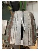
If the correct thickness of packing is available, sure I will use it. I tend to use steel packing because I can then place a bar magnet over the top to secure it before tightening.
