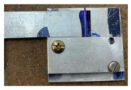
With the reference edge against the guide, I can align my scribed line with the side of the slot and hold it in place with my fingers.
