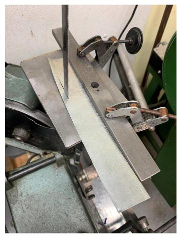
I started by using my tin snips to cut a rough strip. Then I used my belt sander to true up the edge. By pressing a parallel against the edge while looking at the gap with a strong light behind it, I can see gaps as small as 0.0001-inches.
