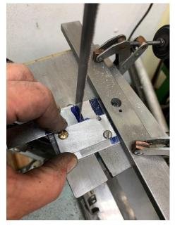
My fingers are at a safe distance from the blade. I pressed the sled against the fence and moved it along to cut the sheet metal.
