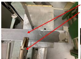
I used 1<sup>1</sup>/<sub>2</sub> inch wide strap. This let me use a Vise-Grip to secure the attachment to the table. The strap is 1/8 inch thick and 18 inches long.
