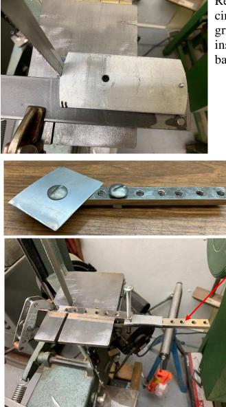
Recently, homemadetools.net had a few interesting circle-cutting attachments. One was for an angle grinder and the other for a plasma cutter. They inspired me to come up with a vertical bandsaw-based arc/circle cutter.
