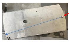
In preparation for sawing an arc or circle, I first drill the center using a #27 drill.
