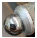
Final alignment of the magnet was performed by dropping a  $\frac{1}{2}$  inch diameter ball bearing into the socket. Then I heated up the part with a hot air gun until the glue started to flow. Next, I pushed the socket down on my bench with the ball bearing on the bottom. This set the magnet in contact with the ball and ball in contact with the socket.
