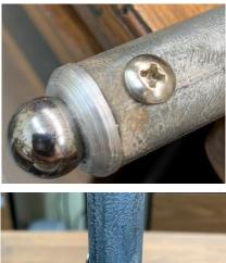
I thought heat glue would hold the socket into the conduit but it did not distribute very well so I drilled and tapped for a 6-32 screw.
