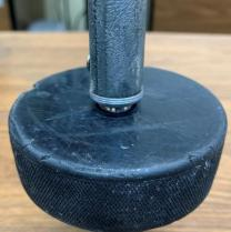
With the conduit roughly vertical, the hockey puck is free to adjust a few degrees and come into full contact with the floor. The magnet is strong enough to hold the hockey puck yet it easily releases if I want to inspect the bottom face. I suspect that swarf will embed itself into the puck and will have to be periodically cleaned.
