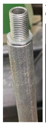
The top of the conduit was intentionally cut about 1 inch short. This let me drop a length of threaded lamp rod with a nut into the top.
