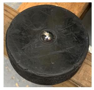
My first step was to chuck up a scrap hockey puck in my lathe. I first drilled it through with a 3/16 inch drill. Then I used a ½ inch ball end mill to drill in about 5/16 of an inch. Then I pressed in a ½ inch diameter ball bearing. It snapped tightly in place. If I had to remove it, I can drive it out through that 3/16 hole.
