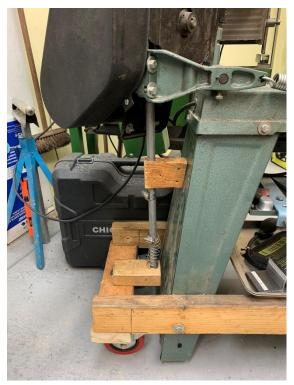
My proof of concept, and possibly my final embodiment, is shown here. When the saw's arm is raised to the vertical position, it pushes down on a length of electrical conduit.
