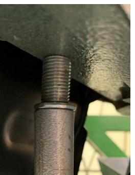
With the arm in the vertical position, I turned the nut until the lamp rod contacted the arm casting. Then, with the arm horizontal, I turned the nut so the lamp rod was about 0.05 inches higher. In this way, the puck will compress into the floor but not raise the rear wheels.
