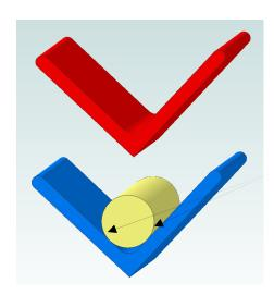
Beevo showed me how you could drop one of the drills into the lower piece of angle and bend strap to angles greater<sup>2</sup> than 90°. The bends are clean and repeatable. Pure elegance!
