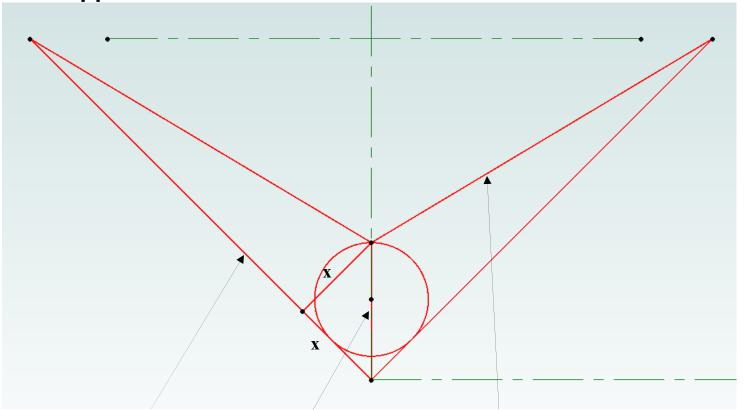
The lower V is the angle stock. / The upper V is the strap bent to the desired angle. The circle is our rod. The vertical line has a length equal to
