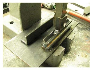
On a recent visit to "Beevo's" shop, I was shown a modification to an arbor press that made bending thin strap easy. A length of ½" angle stock had been welded to a plate with a mating piece of angle attached to the arbor's ram. You can find more details of this machine at:
