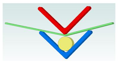
It is not hard to use a "cut and try" method to figure out the drill diameter needed for a given bend angle. But since I enjoy using math in my shop, I came up with a spreadsheet to do the job.
