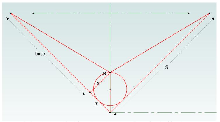
The length of one side of the angle stock is "S". We know that the side of our isosceles right triangle, x, is approximately 0.8536D long so have the base of our larger right triangle
