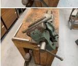
Once in a while, I need to work at other than horizontal. My vise pivots all the way to the jaws being vertical.
