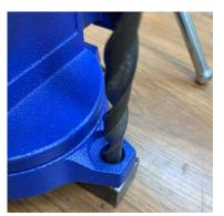
Then I selected a drill that was a close fit to the lug's hole. Using my battery powered drill, I drilled down enough to clearly mark the location.
