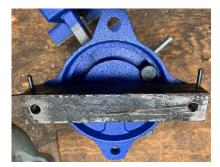
The final step was to drill 1/8 inch holes 0.15 inches from each end. I drilled in about  $\frac{1}{2}$  inch. Roll pins were then pressed in place.
